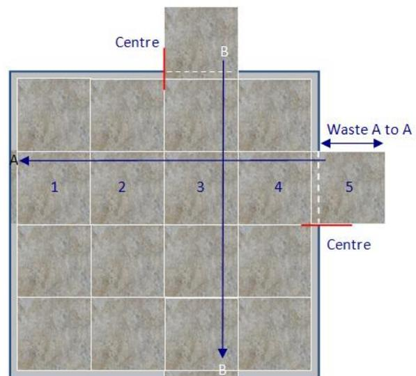
**Illustration 3** is a tile set out from the centre providing a balance at each edge. See **Illustration 4** for the solution that provides a larger cut tile at the edge.
