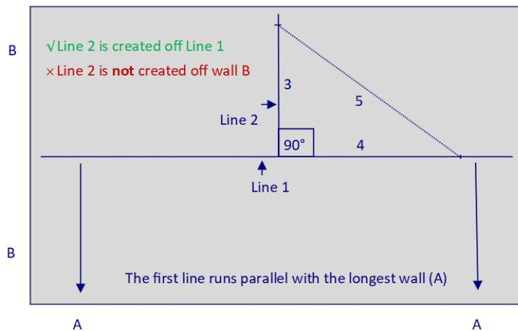
**Step 3** - Repeating the 3-4-5 rule on the opposite of Line 1 side helps with accuracy when setting out larger areas. Points A, B, C should line exactly together when a string line is laid over them.
