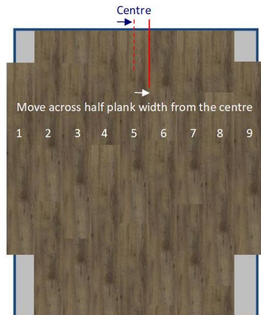
**Illustration 2** is moving a plank set out across from the center by half a plank width. Using the same amount of planks create a wider strip to be cut in at both edges.
