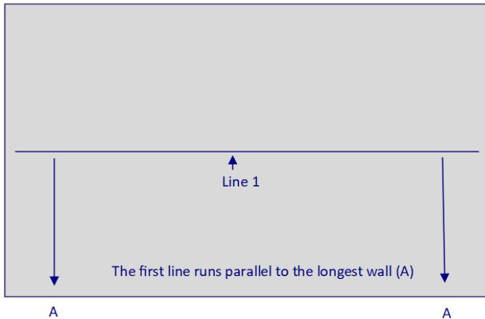
**Step 2**—measure along Line 1 and mark the chosen start point. This may be the centre of the area or will be offset from the centre mark by half a tile width. Create Line 2 off line 1 using the 3-4-5 rule.
