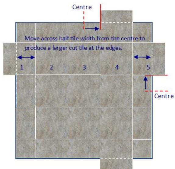
**Illustration 4** shows how moving a tile set out across from the centre by half a tile width increases the size of edge cut tile. The same amount of tiles are used but with a wider edge tile.
