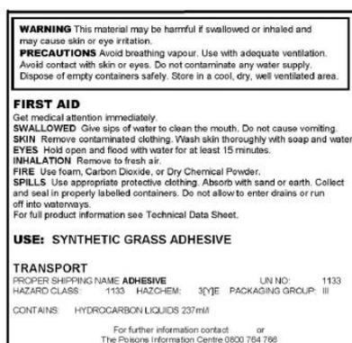
Typical warning label on drum of adhesive.
