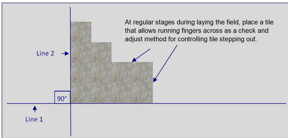
**Illustration 9: Installing tiles in a step form.**
