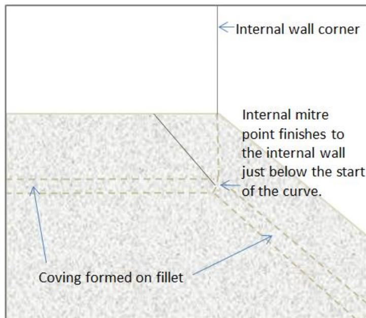
The finishing points should be no lower than 10mm above the floor
