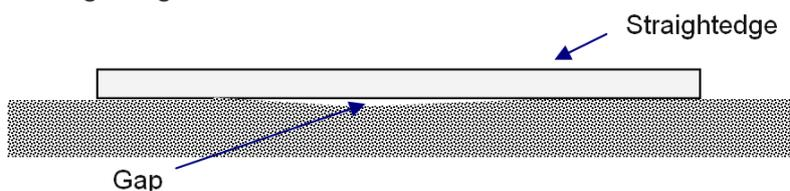
Illustration 7: Checking for gaps beneath a straight edge.
