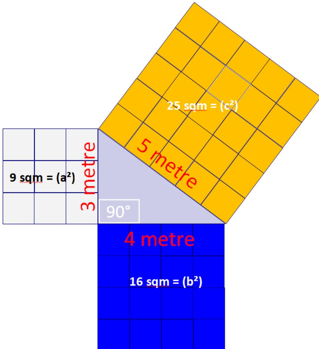
A simple way of applying this to flooring is to think of the 3-4-5 rule in metres. The 3 metre and 4 metre measurements are the right angle and the 5 metre measurement is always the longest side.
