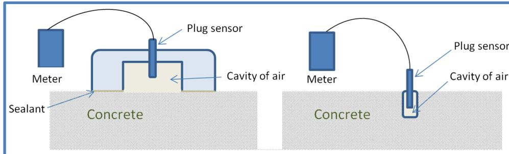
**1. Hood test**—a casing sealed to the concrete surface. A plug inserted into a cavity of air that is readable by a digital meter.
