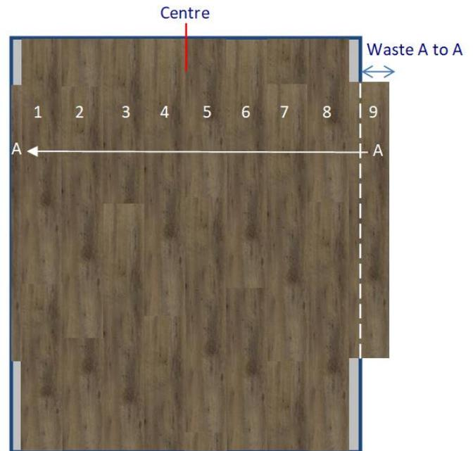
**Illustration 1** is a plank set out from the center. Because of the relationship of the width of the area and plank width, a thin strip is needed to be cut in at both edges.
