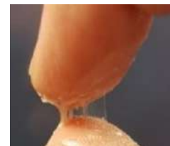
Illustration 2: Depending on temperature and humidity, the adhesive will soon start to develop a tack. Sometimes referred to as 'growing legs'
