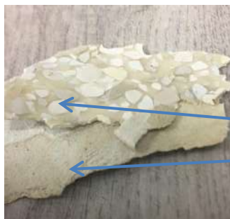
Photo 1 Vinyl wear layer separated from its backing
