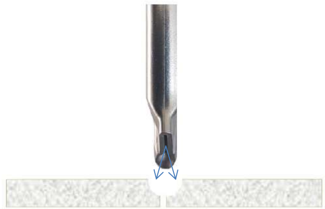
Hot air stream directed into the groove
