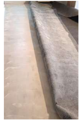
Illustration 3: Adhesive transferred to the carpet backing
